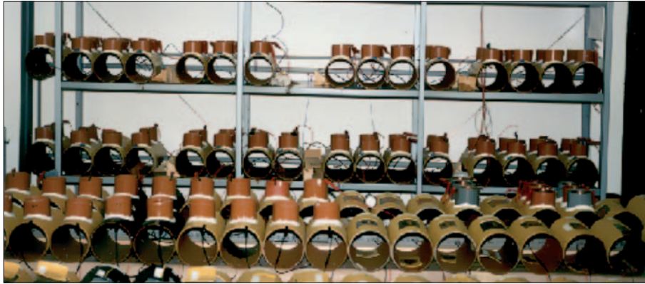
Fig. 7: Test stand for examining cracks in polyethylene coatings
