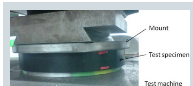
Figure 8: Set up for testing the shear strength
