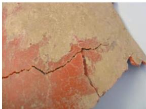
**Fig. 2:** Sintered coating affected by external forces
