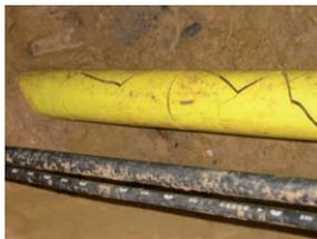
**Fig. 3:** Brittle fracture in an extruded polyethylene coating
