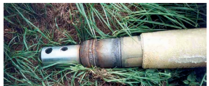
Fig. 13: Steel pipe with jacking head
